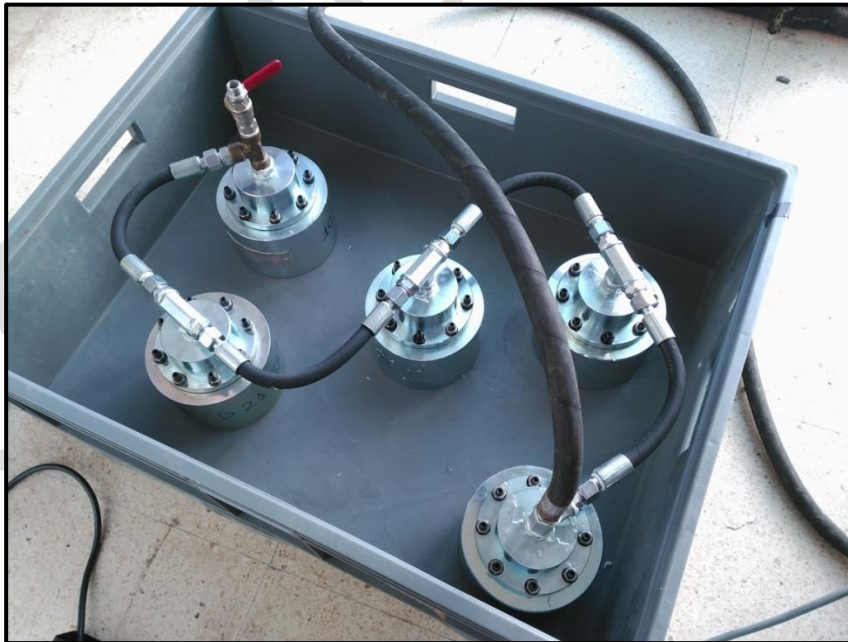
Picture 2 Mounting and execution of tests on five D21x48PS samples
